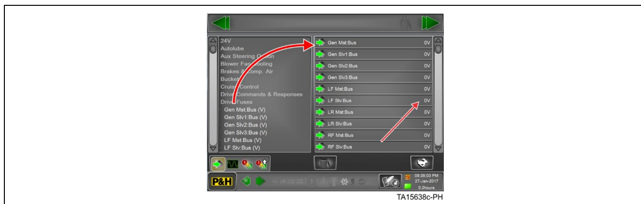
Figure 20. Bus voltage indication
