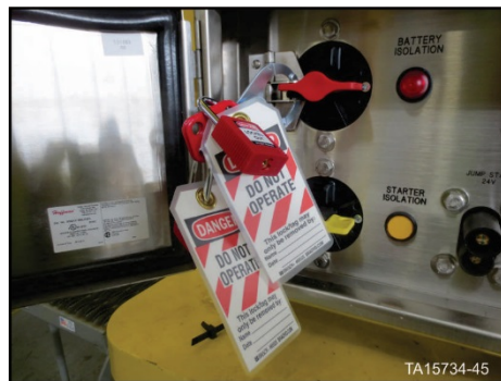
Isolation and Control switches assembly – Battery isolation switch in OFF position with locks in place
