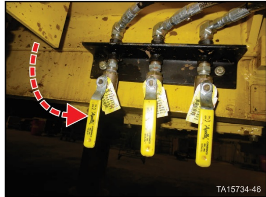
Open air reservoir bleed valves
